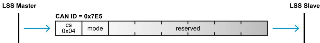
Figure 3-33 CAN communication | LSS commands switch state global
