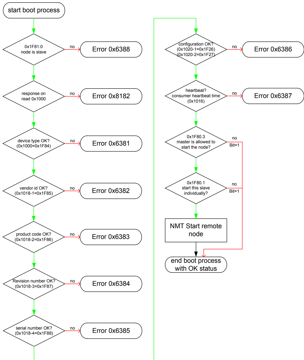
Figure 4: CANopen boot-up procedure slave boot process
